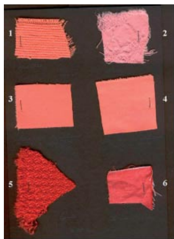
Figure 2. Tintorial tests on 5d performed on: 1) polyester, 2) cotton, 3) polyester \ polyurethane dyed as polyester, 4) polyester \ polyurethane dyed as wool, 5) wool, 6) cotton \ nylon.
